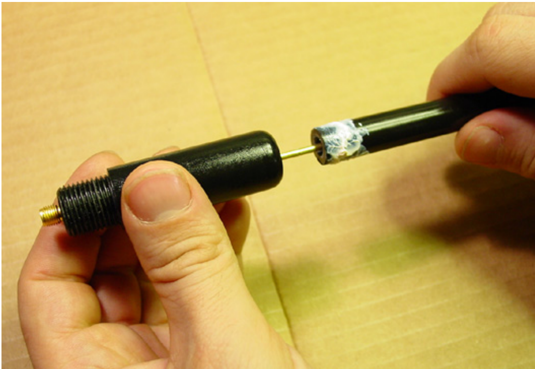
Figure 17. Epoxy applied to radome prior to insertion into threaded mounting component.
