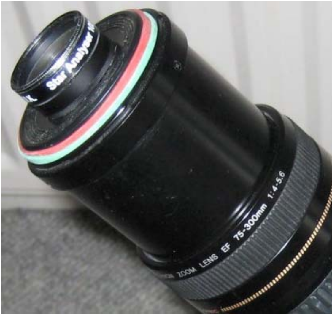
Star Analyser mounted in Lens Cap of DSLR Camera
